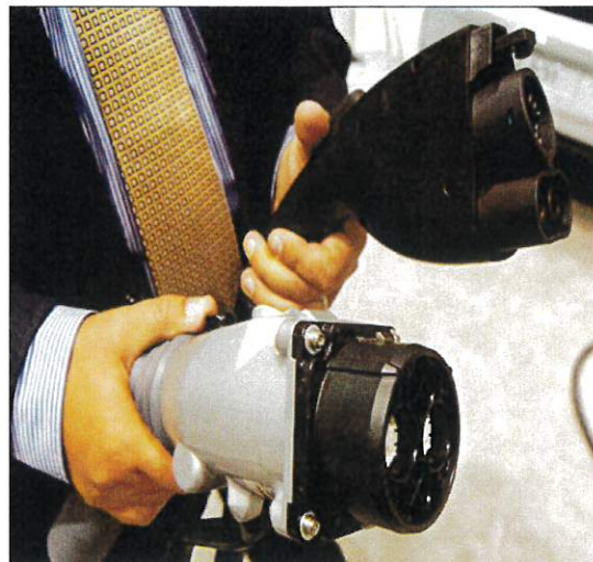
Figure 2: Variations in vehicle charging plugs (Photo Source: VEIC)
